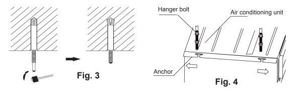
Install the hanger on the indoor unit, as shown in Fig. 4. Install the indoor unit on the ceiling, as shown in Fig. 5.
