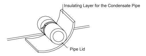
Fig. 13 Thermal Insulation of the Condensate Pipe
