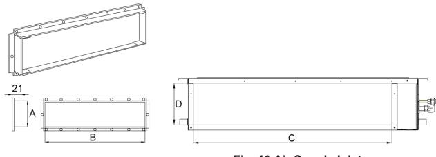
Fig. 9 Air Supply Outlet
